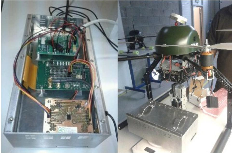
Figure 1: (left) Receiver Hardware mock-up and (right) side by side of a small UAV (JAVISON UX-401L)
