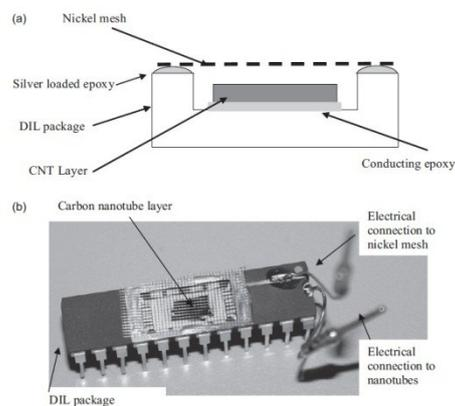
Fig. 2. Dual in line package (DIL) used for carbon nanotube (CNT) testing: (a) schematic showing the location of the nickel extractor mesh at a distance of ~1 mm from the upper surface of the CNT layer and (b) photograph of the DIL package showing the external mesh, fixed to the package manually using conductive epoxy. The individual electrical connections to the mesh (top of the package) and nanotubes (base of the package) are also indicated.
