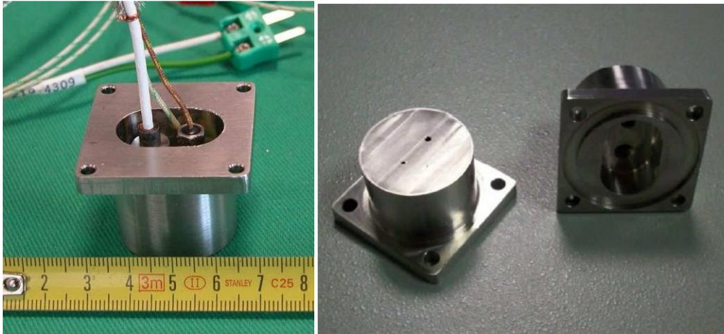
**Fig. 1 Example of unit: EXPERT Streamlined Sensor Unit (2 thermocouples, 1 pressure sensor)**
