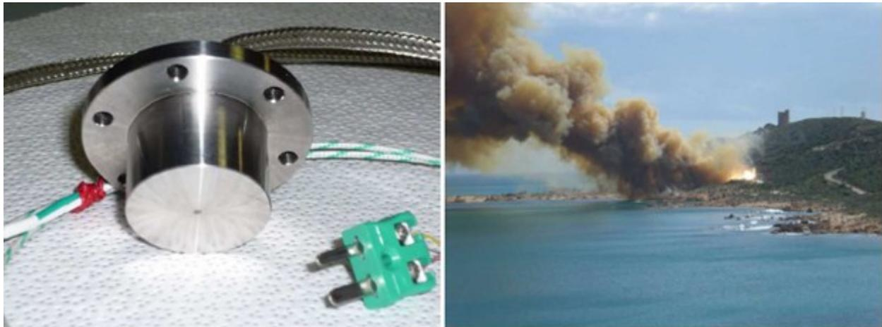
Fig. 3 Example of unit: heat flux units used for VEGA Zefiro 9 solid propellant thruster
