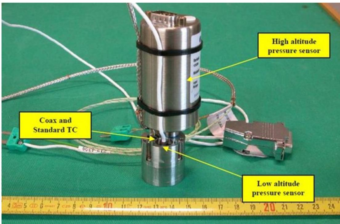
**Fig. 2 Example of unit: EXPERT baseline Sensor Unit (1 thermocouples, 2 pressure sensors)**
