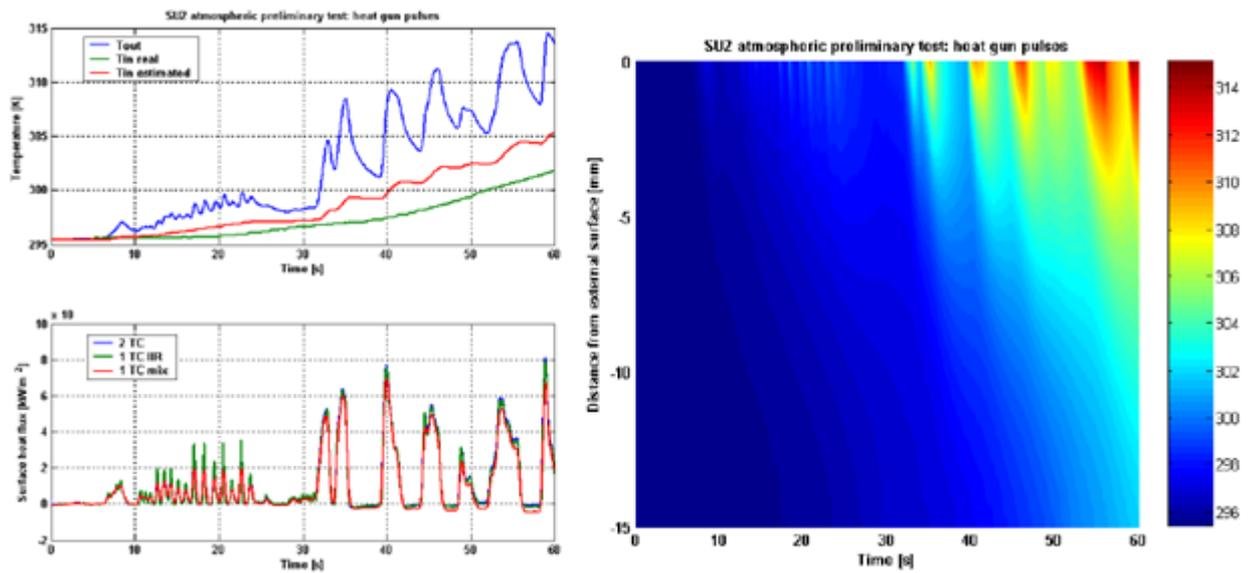
Fig. 4 Example of calibration run: temperature and surface heat flux history (left) – internal temperature history (right)
